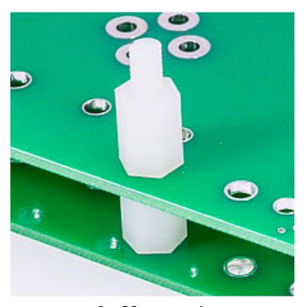
a **standoff** is used to raise PCBs off of a surface
